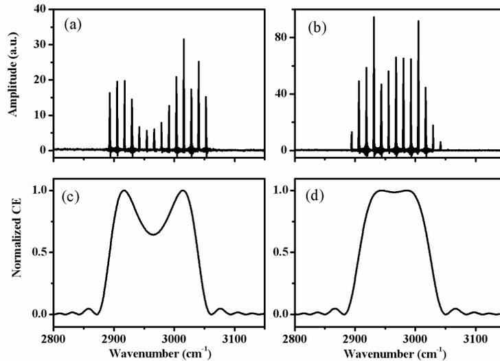
Fig. 4. Measured output spectrum of the DFG laser source with (a)  $T = 73.5^{\circ}\text{C}$  and (b)  $T = 75^{\circ}\text{C}$ , and calculated normalized conversion efficiency with (c)  $T = 73.5^{\circ}\text{C}$  and (d)  $T = 75^{\circ}\text{C}$ .
