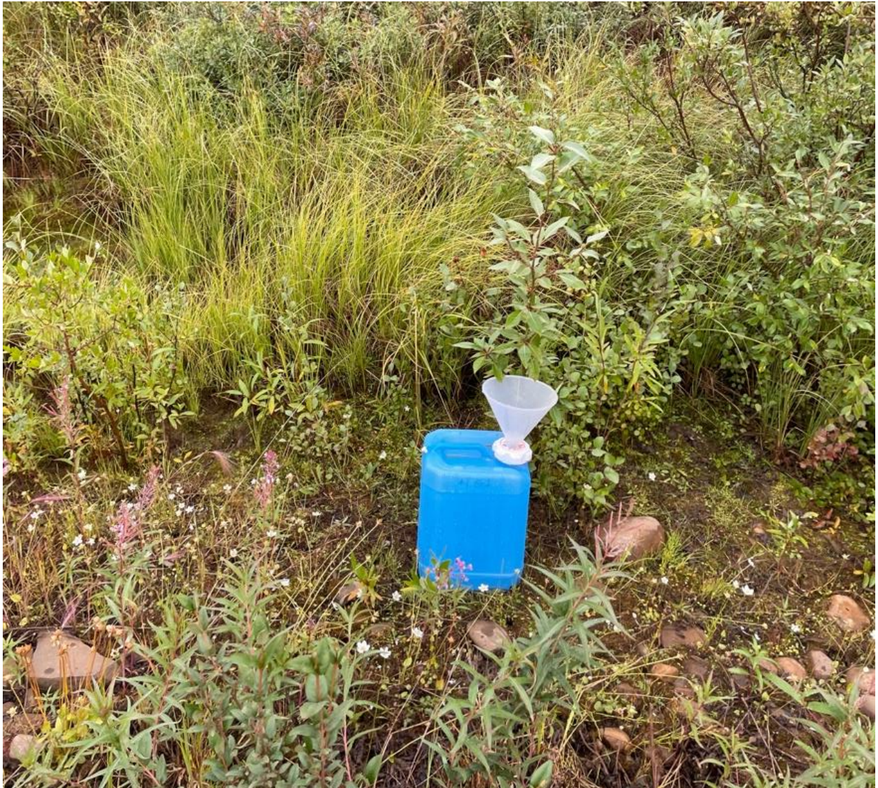
Figure 2.2. Dust collection trap used to measure how far from the road dust was travelling across the landscape.
