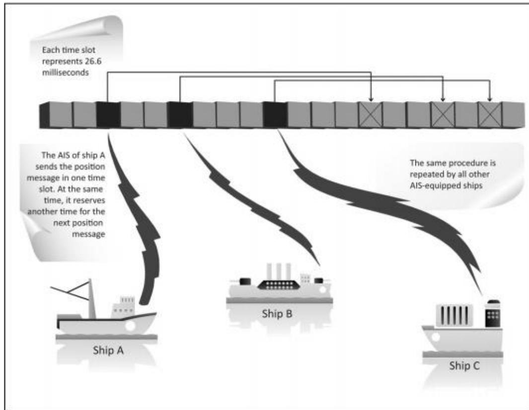
Figure 2.1: SOTDMA protocol for reporting timeslots. Variable timeslots exist depending on the ships speed and where it is going. (Ball, 2013)
