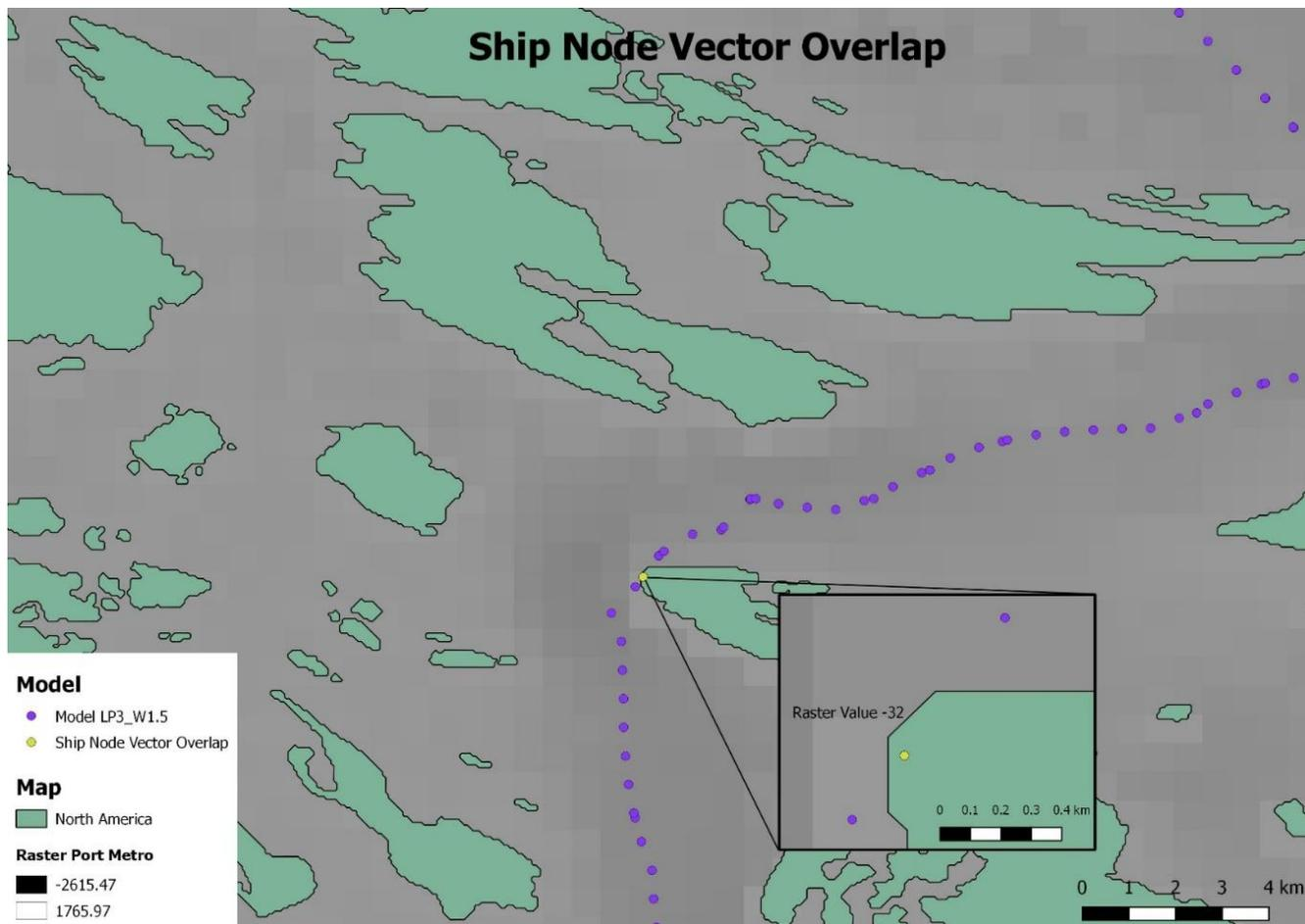
Figure 2.6: Ship node vector overlap. Due to the scale of various maps, nodes can appear on land.
