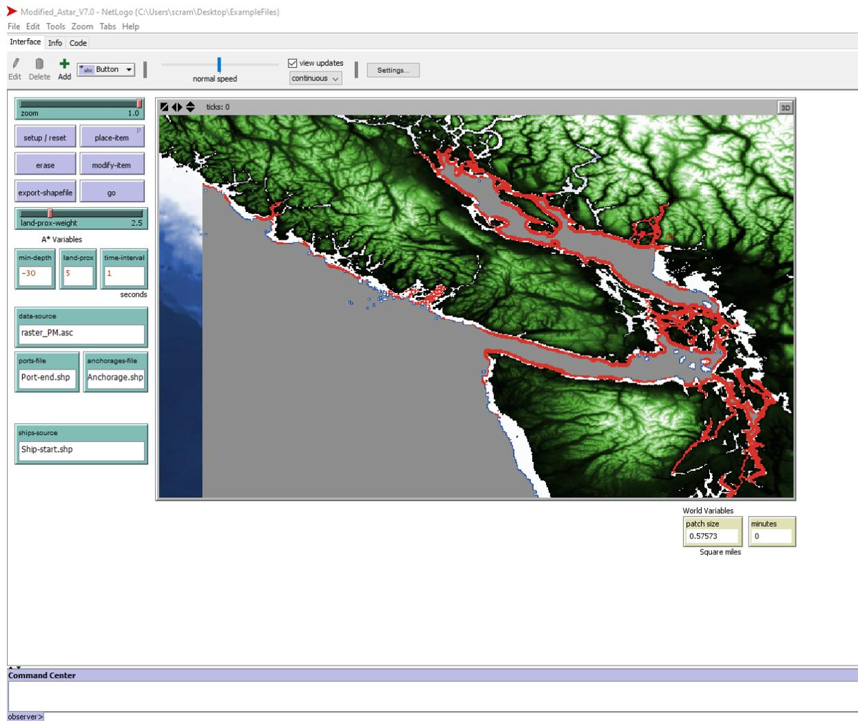
Figure 3.2.4 LP5 path finding algorithm example. The number of red pixels indicate how many nodes in the waterway are being affected by the LP distance.
