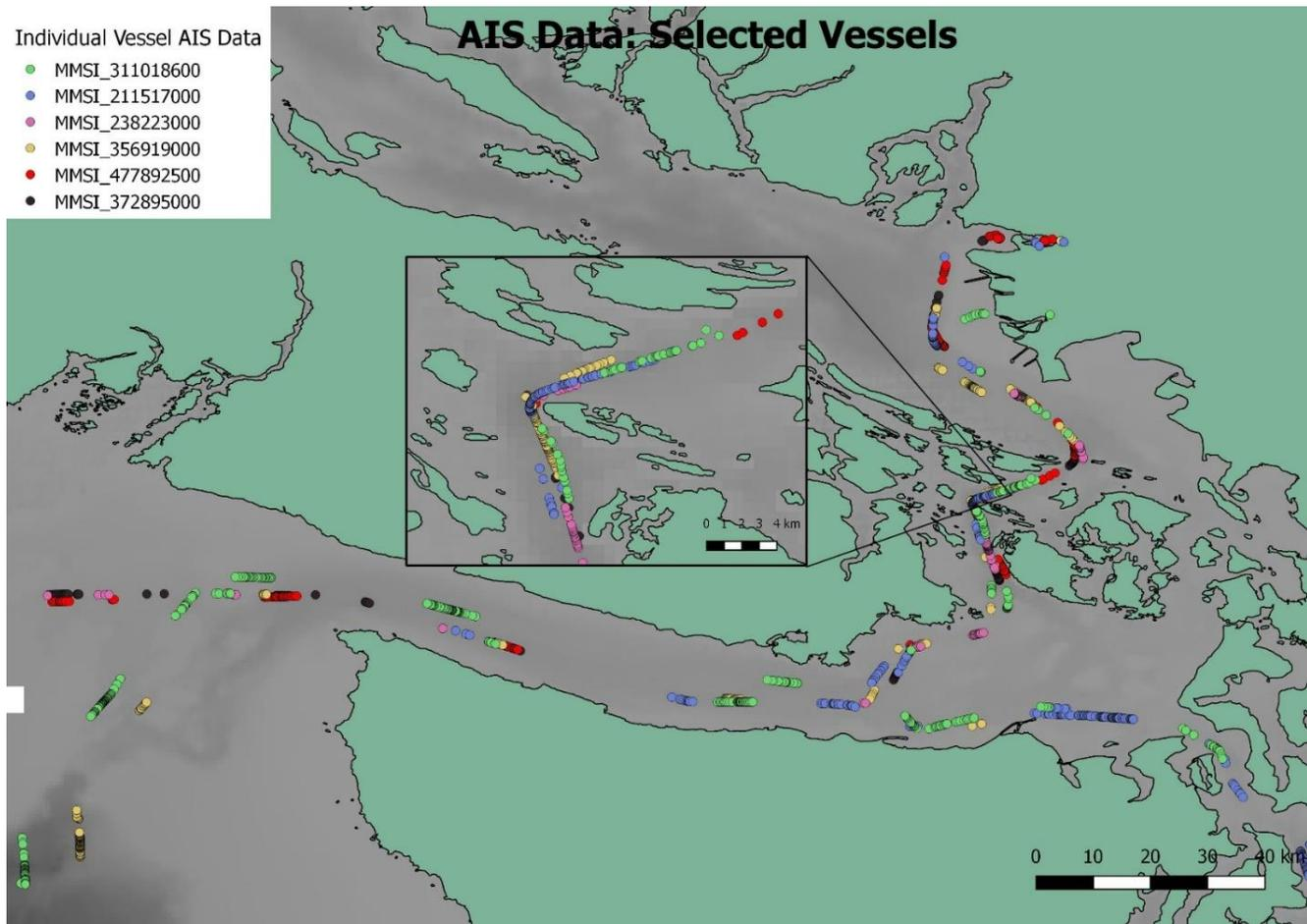
Figure 2.8: AIS Data: Selected Vessels. Manual Selection of several ships from the AIS data. Highlights the sparse nature of AIS data recordings.
