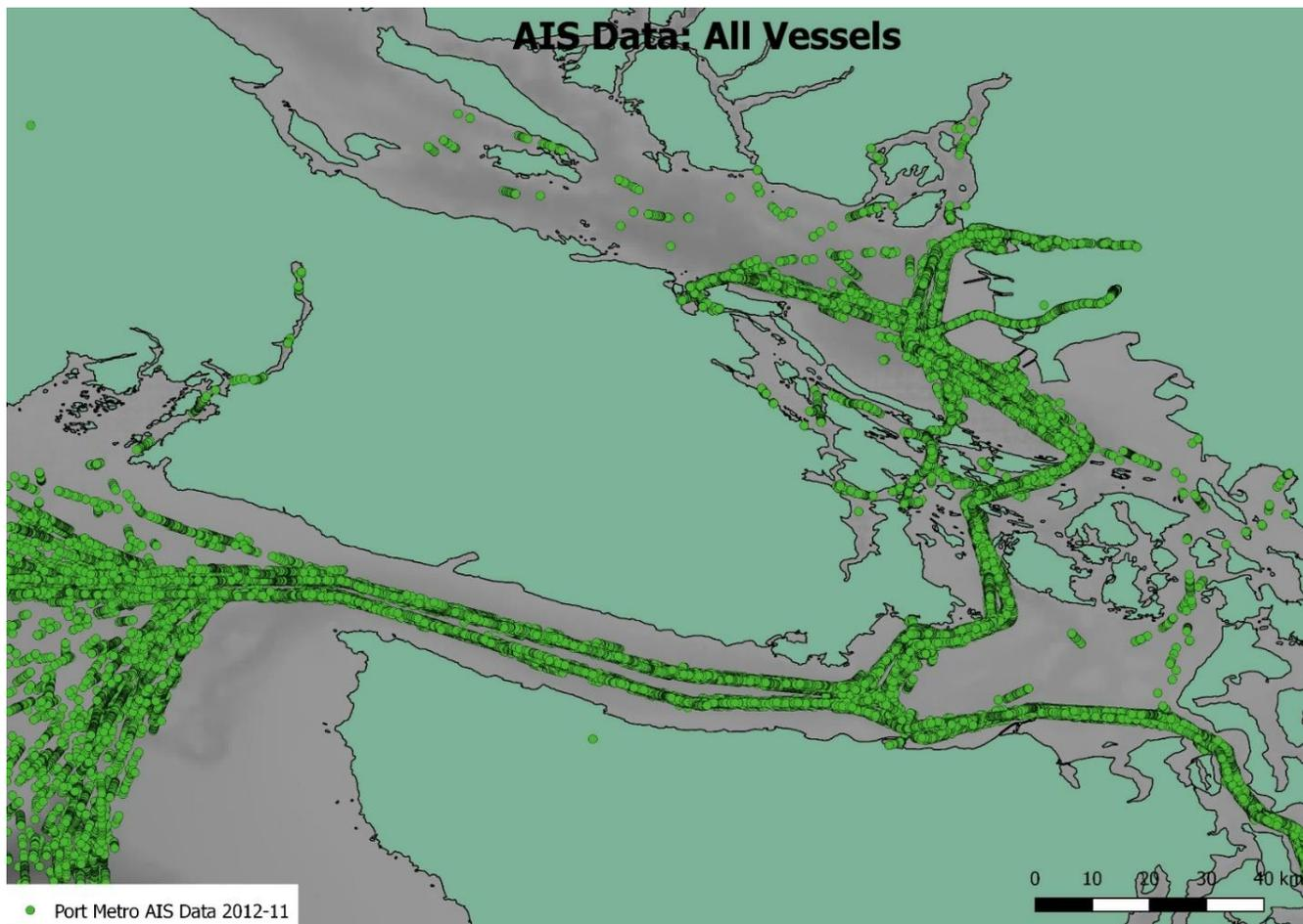
Figure 2.9: AIS data: all vessels. This shows how much data was included in the original selection of AIS messages. Clean up was necessary to make sense of the overabundance of information.
