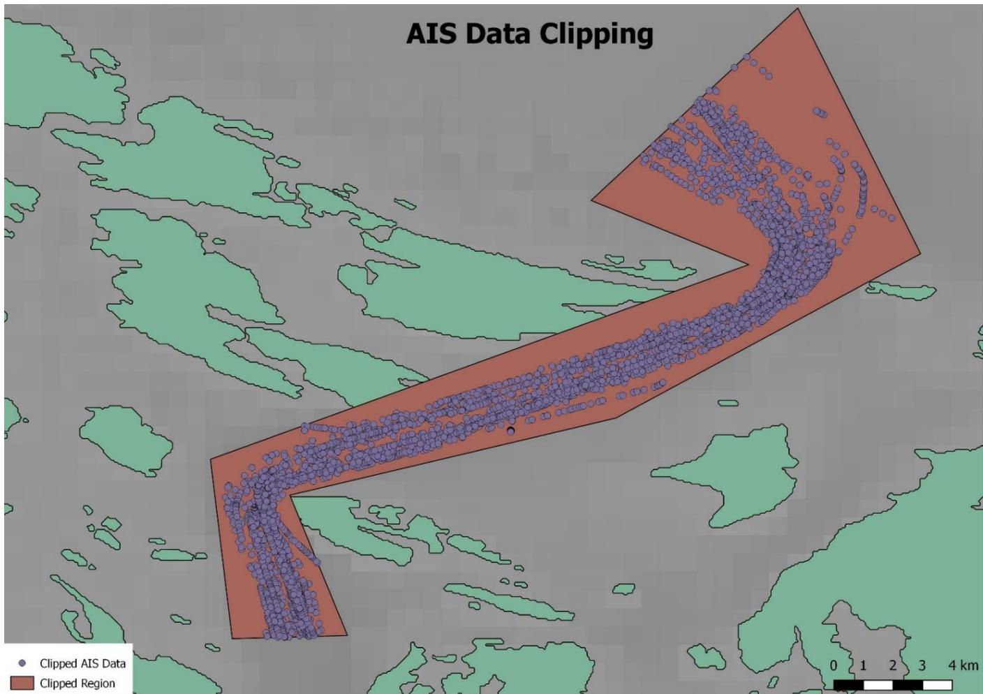
Figure 2.10 Data clipping of raw AIS data (before manual removal of erroneous points)
