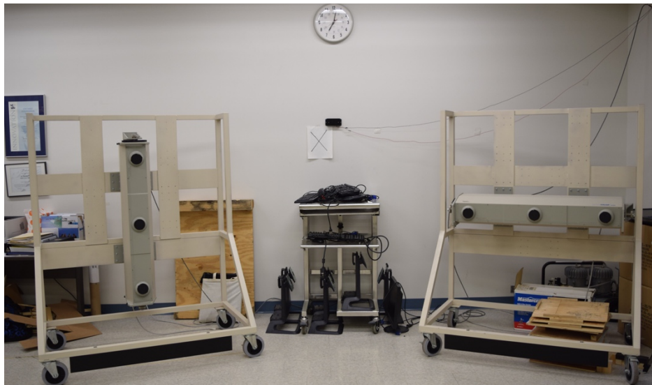
Figure 5. OptoTrak 3020 Motion Analysis Systems: (Left to Right: Vertical and horizontal configuration).
