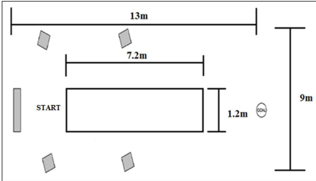
**Figure 8-** The experiment took place in a 13m by 9m space, with full lighting. Within this space was the 7.2m by 1.2m pathway which contained the raised rock climbing holds. Five Optotrak cameras were positioned in a semicircular formation in order to capture full-body kinematics of the participants throughout the entire pathway.
