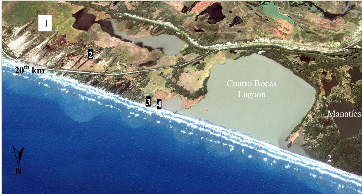
Figure 21. Image taken on January 22<sup>nd</sup>, 2013 showing 1. stabilized dunes at the 20<sup>th</sup> km with dunes length up to 1.3 km. 2. Overwash channels approximately parallel to the direction of the dunes. 3 and 4. Location of overwashes detailed in figure 30.
