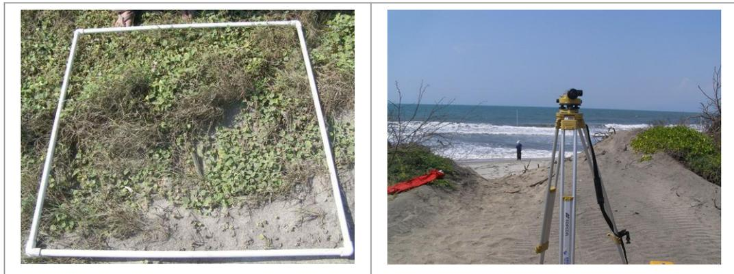
Figure 13. 1 m<sup>2</sup> quadrat to identify and quantify vegetation (left) and topographic profile along dunes, the latter using an AT G6 Topcon level (right).
