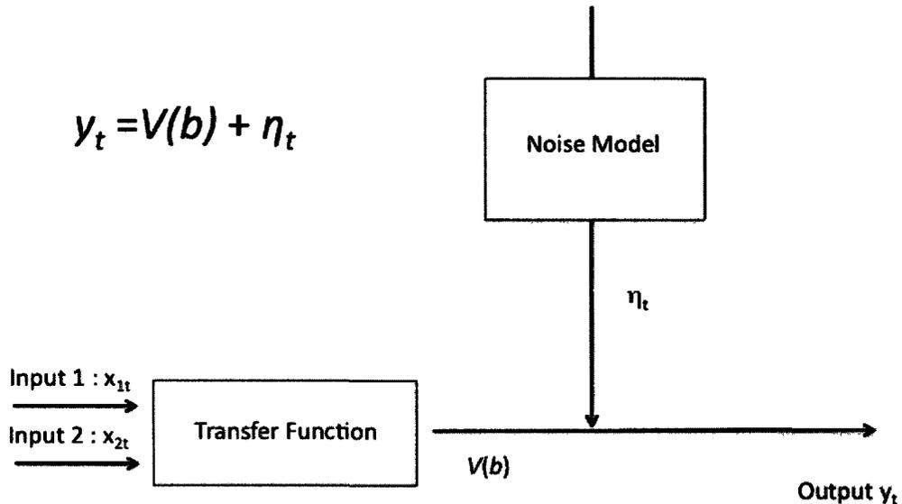
**Figure 6 Schematic representation of a transfer function model with multiple inputs (Helfenstein, 1996)**
