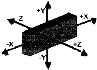
**Figure 4 Accelerometer showing axis orientation and values (+ or -)(c) Sean Doherty, 2006**
