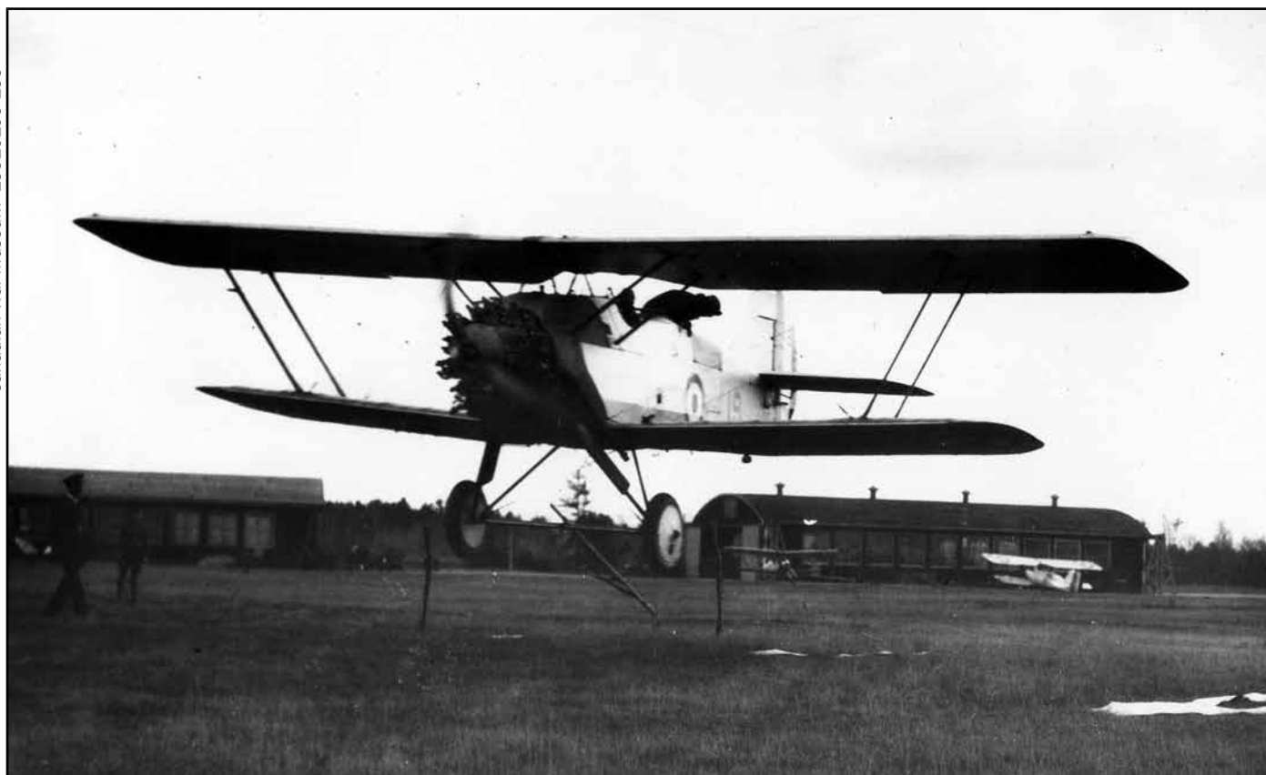
The Armstrong Whitworth Atlas was a purpose-built army co-operation aircraft based on First World War experience. Here an Atlas skims low over an airfield to practice a message snatch. Note the observer leaning over the side of the aircraft.
