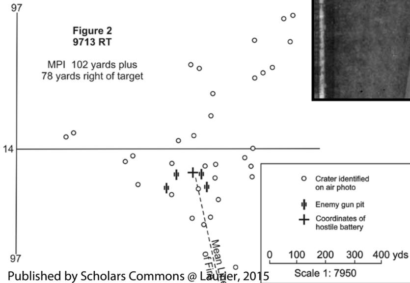
**Left:** This figure shows a plot of the artillery shells directed at the German battery. It was found that the mean point of impact (MPI) was 102 yards past and 78 yards to the right of the target. Only 11 shells of 112 fired fell with a 100 yard box centred on the target.
