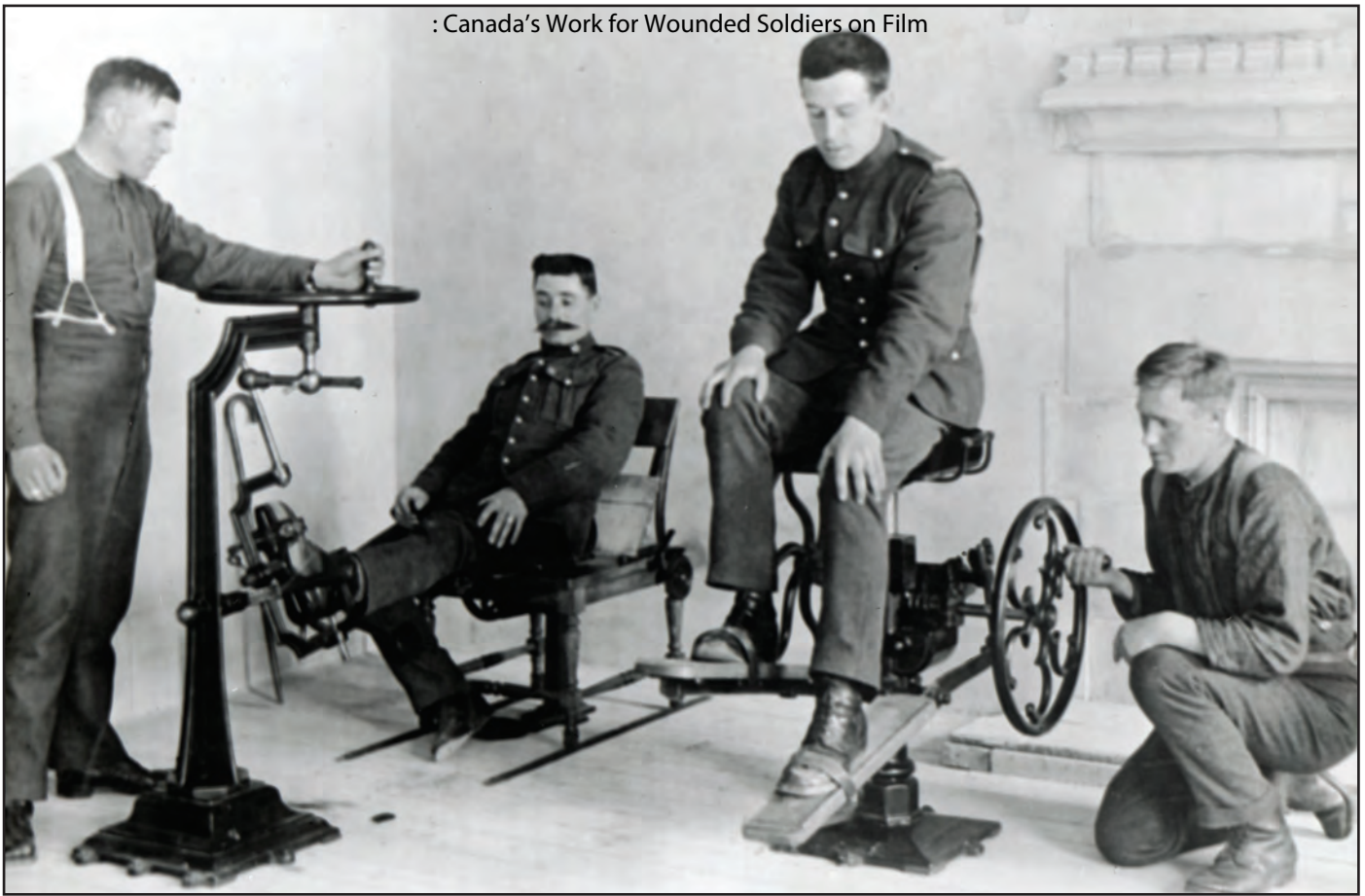
Veterans work on their rehabilitation using Zander exercise machines, precursors to the equipment found in fitness clubs today that use resistance and weights to exercise specific muscles groups.
