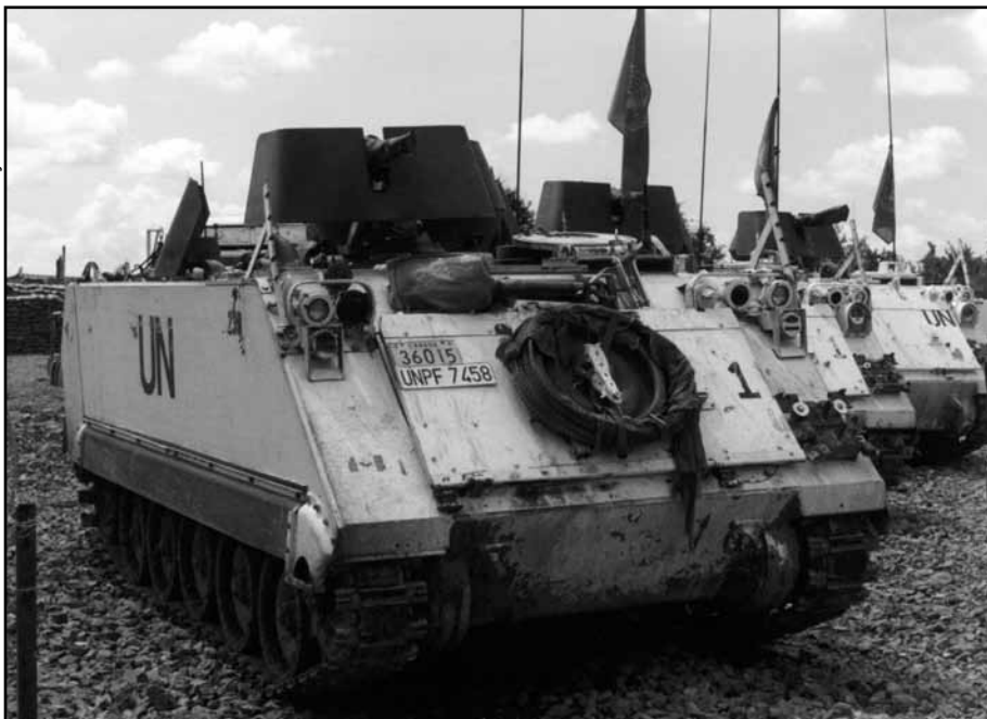
Bottom: Canadian M113A2 with Armoured Cavalry (ACAV) shields fitted, Bosnia 1993. These shields, which were first used by the US military during the war in Vietnam, were designed to give limited frontal protection when firing the crew commander's forward mounted M2 .50 cal Heavy Machine Gun and the two side pintal mounted Light Machine Guns. Many of the Canadian UNPROFOR M113s in The Former Yugoslavia had these shields installed while in theatre in order to provide added crew protection when patrolling the volatile front lines between the warring factions.
