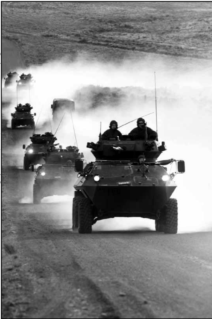
Top: Three variants of the Armoured Vehicle General Purpose (AVGP), a six-wheeled vehicle, were introduced into Canadian service in 1976. (l. to r.) the Cougar fire support vehicle, the Grizzly infantry carrier, and the Husky maintenance vehicle.
