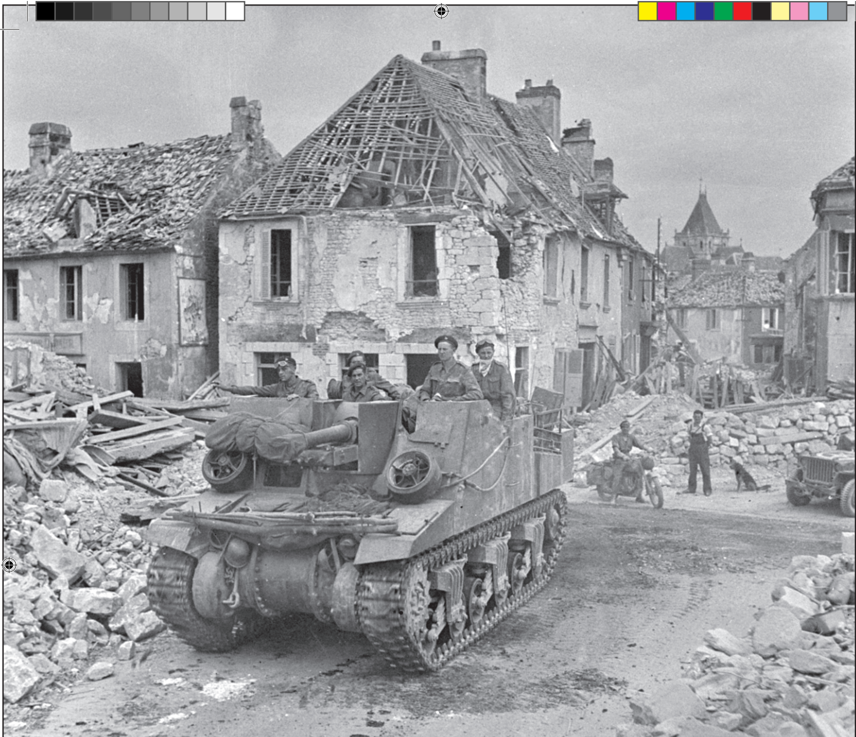
A Sexton gun detachment on the move through a battle-damaged town. Two spare road wheels are mounted on the front armour, along with stretchers, and what appears to be a pair of war trophies – captured German steel helmets.
