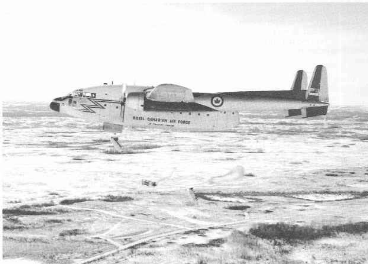
CI 19 dropping cargo through a bottom hatch.
