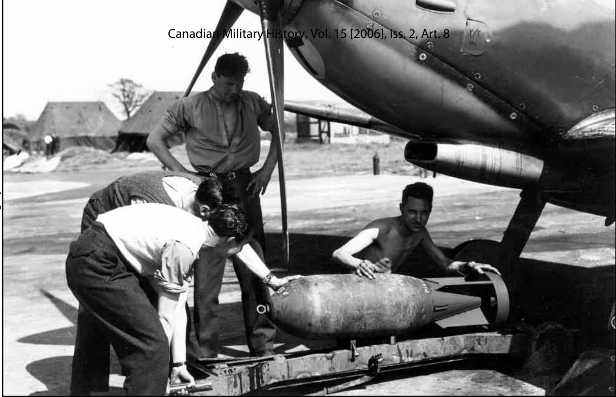
A Supermarine Spitfire of 2nd Tactical Air Force is bombed up with a 500-pounder in preparation for a dive-bombing attack in France.
