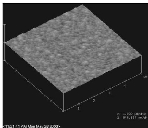
**Figure 1.** AFM image of the Ta/Si wafer surface following 10 min of galvanic Cu deposition from 6.1 M  $\text{NH}_4\text{F}$ , 0.01 M  $\text{CuSO}_4$ , 0.01 M ascorbic acid, and 7.5 M  $\text{CH}_3\text{OH}$ , with Ar deaeration.
