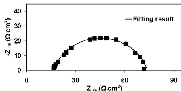
**Figure 4.** Nyquist representation of the steady-state impedance for a Ta electrode at  $-700$  mV SCE in 2.5 M HF.
