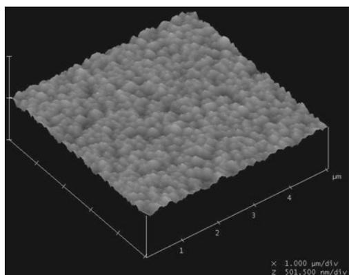
**Figure 2.** AFM image of the Ta/Si wafer surface following 10 min of electroless Cu deposition from 0.05 M  $\text{CuSO}_4$ , 0.6 M  $\text{NaOH}$ , 0.067 M  $\text{Na}_4\text{EDTA}$ , and 0.01 M  $\text{HCOH}$ , with Ar deaeration.
