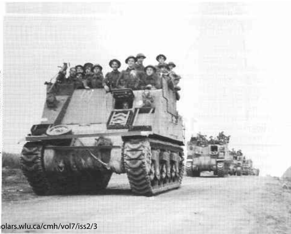
A column of "unfrocked Priests"-M7 SPs converted to armored personnel carriers - with troops from the 51st Highland Division, 7 August 1944
