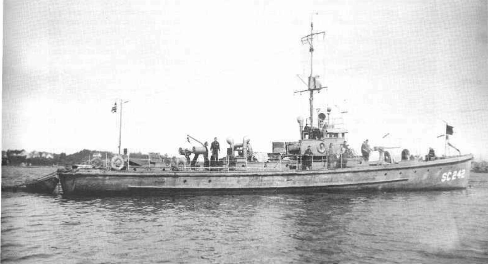
SC 242 - One of the six 110-foot wooden American submarine chasers that operated under RCN control in May-November 1918. SC 242 was part of the division that ran fast escort missions from Sydney. In addition to a stern depth charge chute, she carried a "Y" gun, which can be clearly seen on the quarter deck, to fire charges off both beams. Forward is a 6-pounder quick-firing gun.
