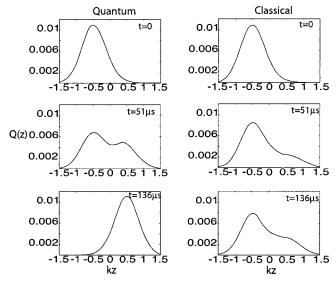
FIG. 3. Reduced Q distribution in position Q(z), at different times in the quantum versus classical evolution. The quantum distribution oscillates between wells, while the classical distribution remains mostly on the left side, with a portion equilibrating between the wells.
