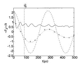
FIG. 2. Predictions of mean magnetization dynamics. Ideal quantum theory: two-level Rabi flopping (dashed dotted); Ideal classical theory: localized at positive  $\langle F_z \rangle$  (solid); Experimental: (circles) with a damped sinusoid fit. The upper bound on the break time between quantum and classical dynamics is  $t_{\hbar}^> = 89 \ \mu s$  (see text).
