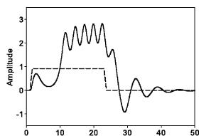
FIG. 10. Numerical simulation results for Q=2.66 showing the response of a junction to a bias pulse (dashed) with equivalent parameters to compare with the experimental data shown in Fig. 9.
