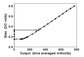
FIG. 6. Hysteretic characteristic from the electronic analog (oscilloscope data). The vertical scale indicates only the magnitude of the applied bias voltage. This response is equivalent to the dc I-V characteristic of a Josephson junction.
