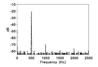
FIG. 5. FFT spectrum (taken from the TDS 2022 oscilloscope) showing of the spectral content of the output from the six diode sine converter when the input triangle wave amplitude is optimized. The fundamental in this case is at 500 Hz.
