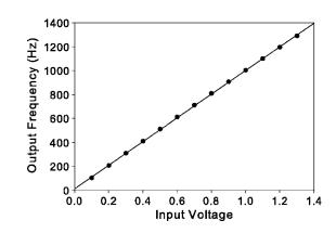
FIG. 3. Calibration of the VCO. From the slope, the conversion factor k is found to be 987.6 Hz/V.
