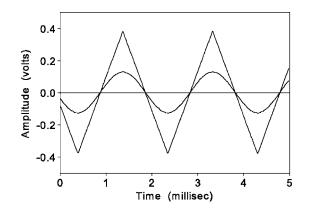
FIG. 4. Oscilloscope data showing the action of the six diode sine converter.
