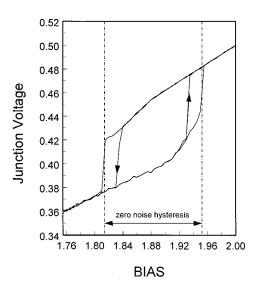
FIG. 9. Hysteresis loop in the current voltage characteristic for the junction, with and without noise. For the computational grid used here, the noise amplitude  $\sigma$ =0.10 corresponds to  $kT/E_J$ =1.4×10<sup>-5</sup>.
