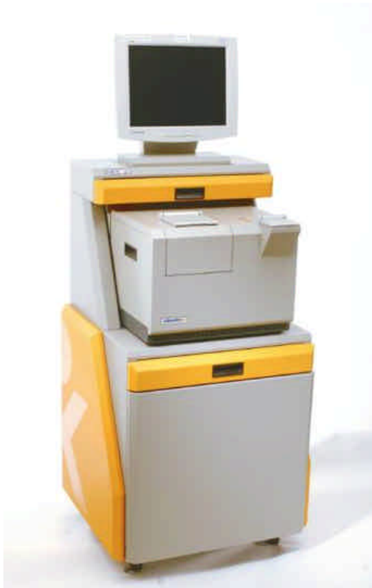
Figure 1 (left): NEC's LS21™ Live Scan Workstation. Law enforcement agencies can capture, archive, search and exchange fingerprints, palm prints and mugshots from this workstation.
