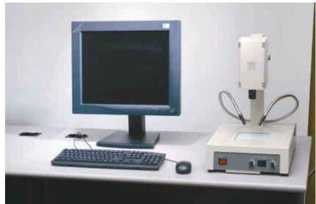
Figure 2 (above): A latent fingerprint workstation by NEC. Allows law enforcement personnel to scan latent prints for examination and archive and exchange prints within an AFIS program.
