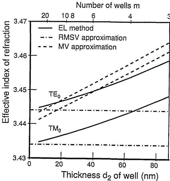
Fig. 1. Effective index  $N$  as a function of well thickness  $d_2$  and the number of wells  $m$ . The other data are  $d_1 = d_2$ ,  $n_a = n_s = n_1 = 3.36$ ,  $n_2 = 3.62$ ,  $\lambda = 875$  nm, and  $d_t = 440.7$  nm.
