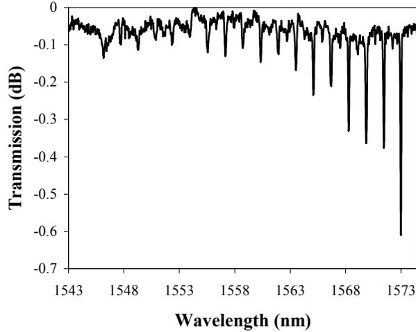
Fig. 4 The transmission of a 20 mm long MFBGs shows the principal modes coupling.
