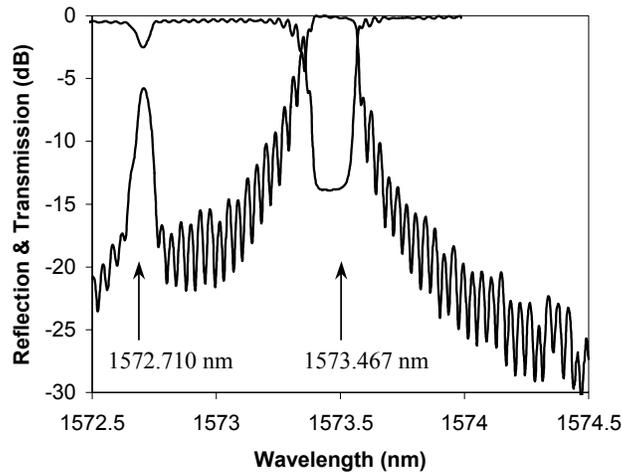
Fig. 2. The transmission and reflection of a 20 mm long multimode fiber grating
