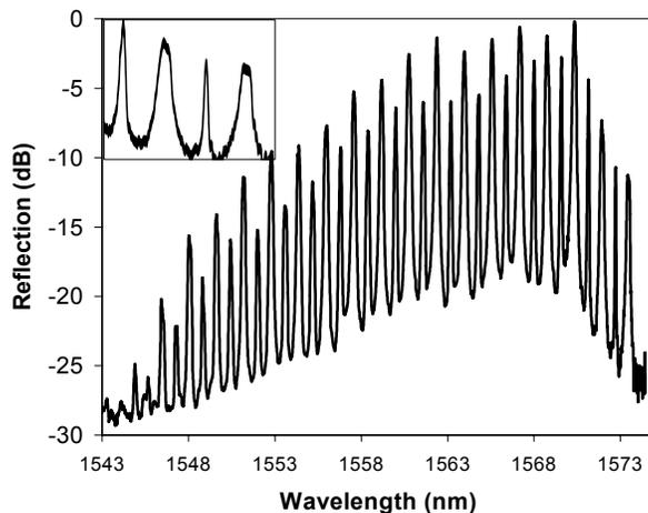
Fig. 3. The reflection spectrum of a 20 mm long MFBG. Two groups of reflections correspond to 18 principal modes (strong) and neighbouring cross coupled modes (weak).
