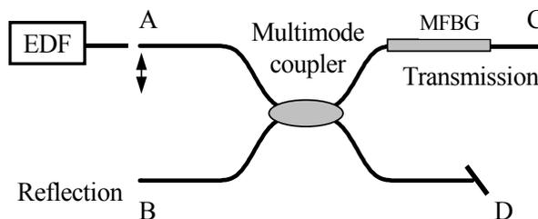
Fig. 1. Experimental measurement of multimode fiber gratings
