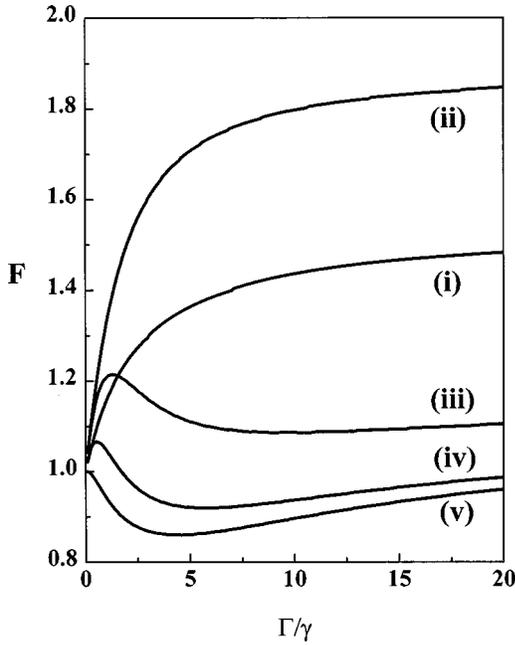
FIG. 4. Fano factor versus pump rate for various values of  $\beta$ . For all plots,  $\gamma_f/\gamma=10.0$  and  $\kappa/\gamma=0.1$ . (i)  $\beta=0.1$ , (ii)  $\beta=0.3$ , (iii)  $\beta=0.5$ , (iv)  $\beta=0.7$ , and (v)  $\beta=0.9$ .
