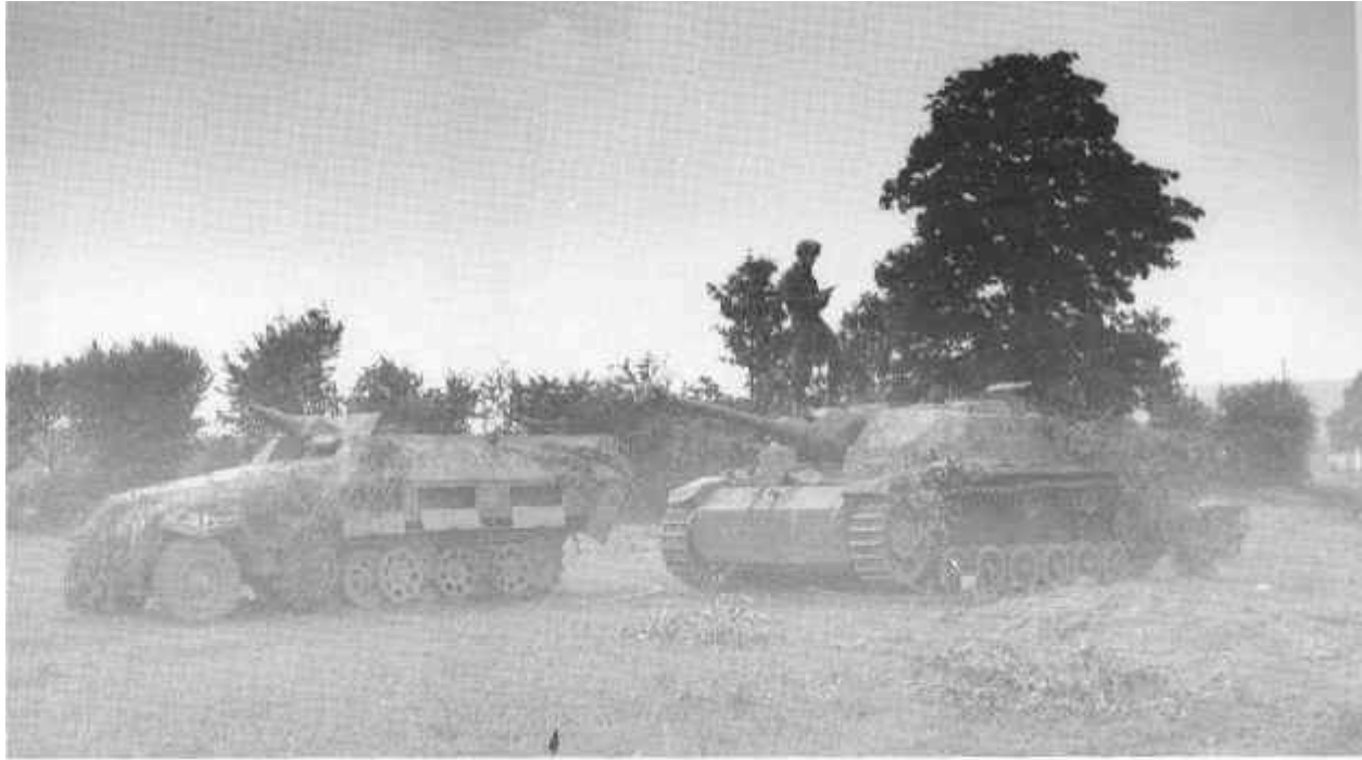
Captured German armour: Sd.Kfz 251/9 halftrack with 7.5 cm gun (left) and a Stug III.
