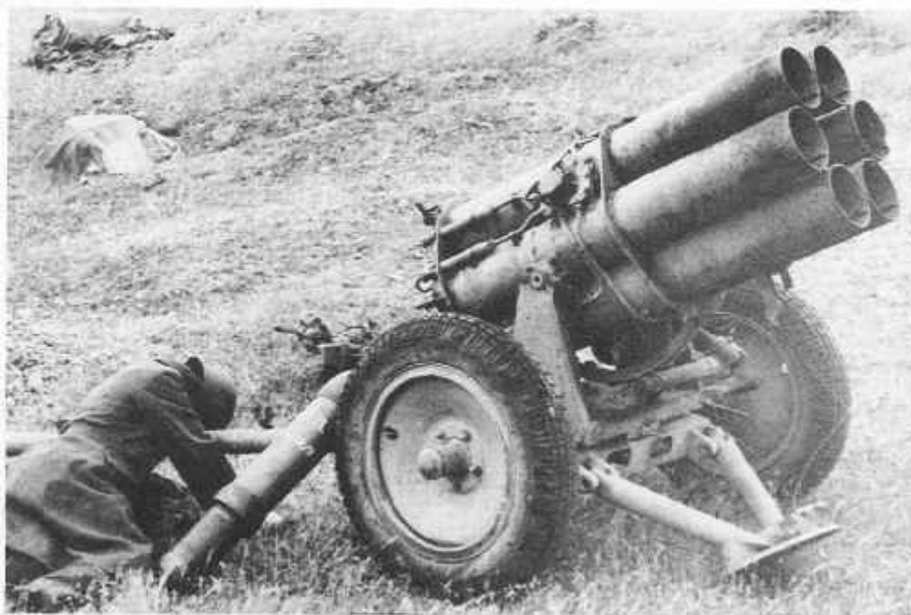
A German Nebelwerfer six-barrelled rocket projector. Allied troops called it "Moaning Minnie" because of the sound of its projectiles.
